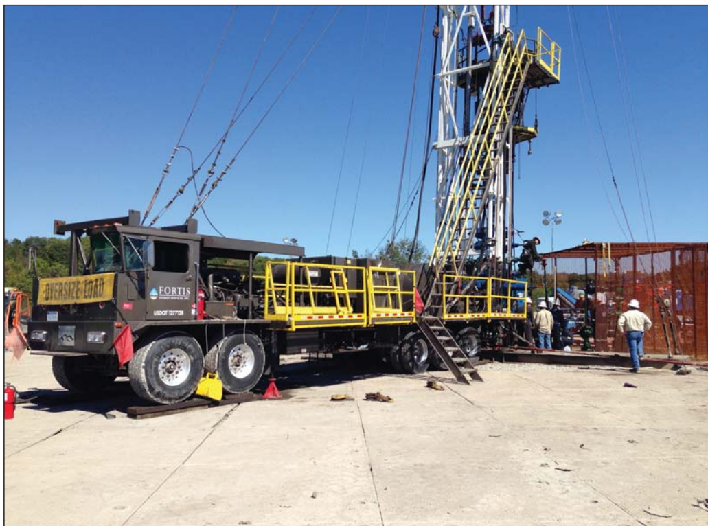
Fortis Rig 1065 completing a well in the Utica.
