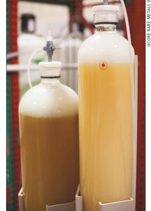
Ligands, such as the ones in these bottles, are molecules or ions that bond to metals. The SuperLig-One pilot plant uses ligands designed specifically to bind with the desired rare earth elements suspended in a solution derived from the Bokan Mountain deposit in Southeast Alaska.
