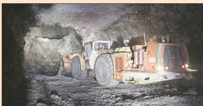
A remotely operated semi-autonomous long-haul dump loader operating during shift changes is helping to boost production at Hecla's Greens Creek Mine in Southeast Alaska.
