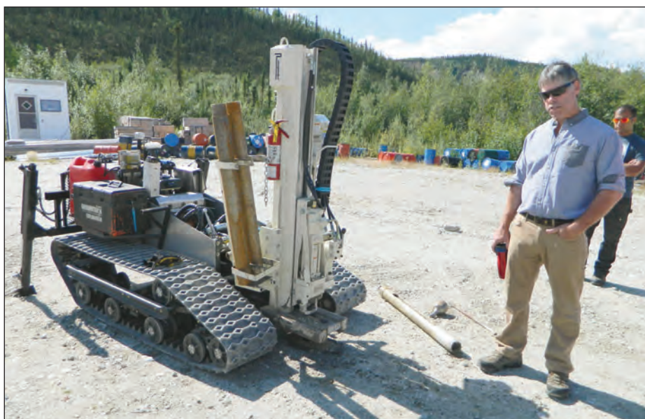
Yukon Territory prospector and entrepreneur Shawn Ryan pauses during an inspection of the newly modified GTProbe® mechanical sampler that an increasing number of junior mining companies are employing for early-stage exploration programs in Yukon Territory. The vehicle, assisted by a three-person crew, can obtain up to 57 soil samples per day over 200-300 meters for a fraction of the cost of conventional methods. Ryan is a co-developer of the device.
