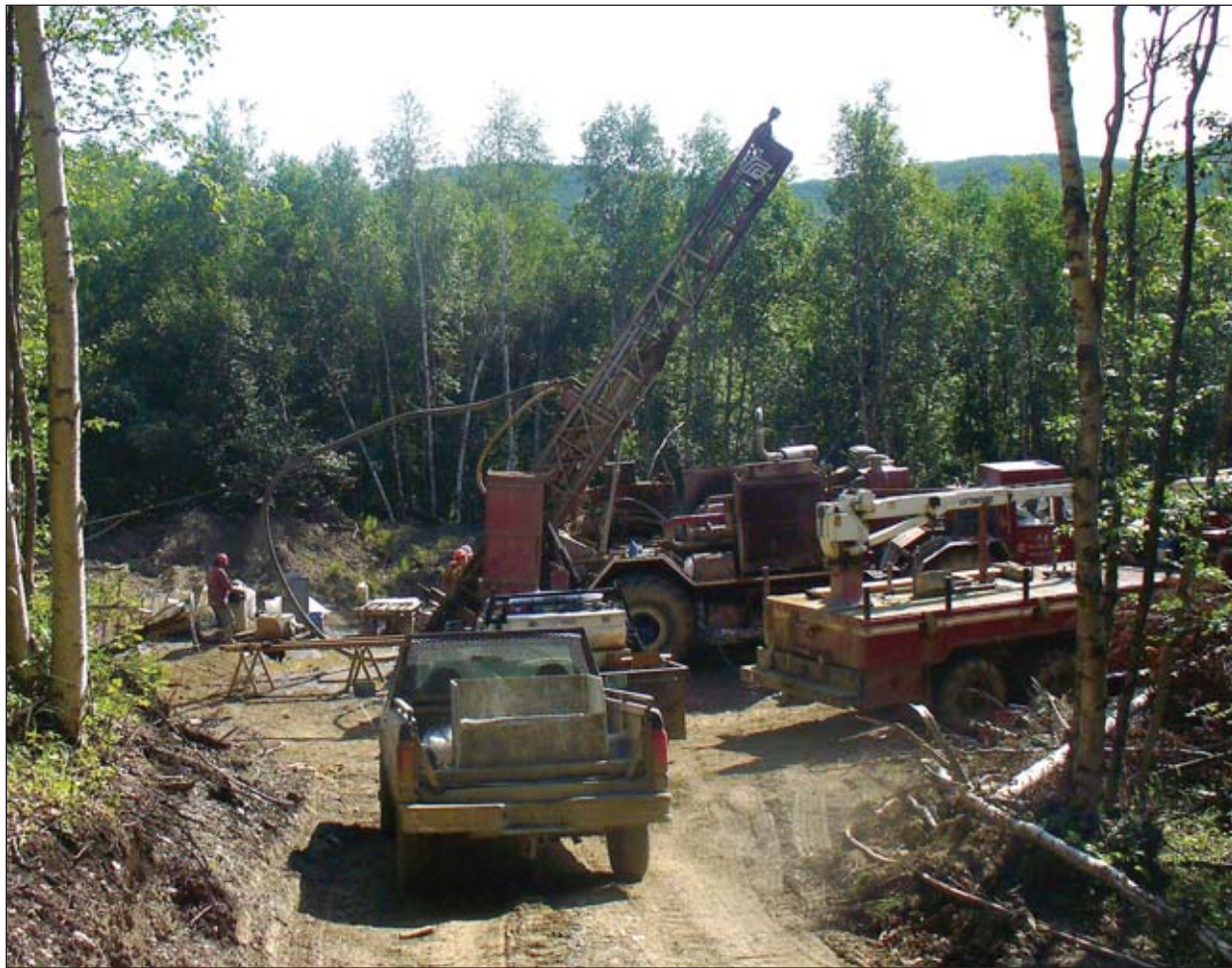
A reverse circulation rig drilling hole MK-RC-0188 into the Sunshine zone at International Tower Hill Mines' Livengood project.
