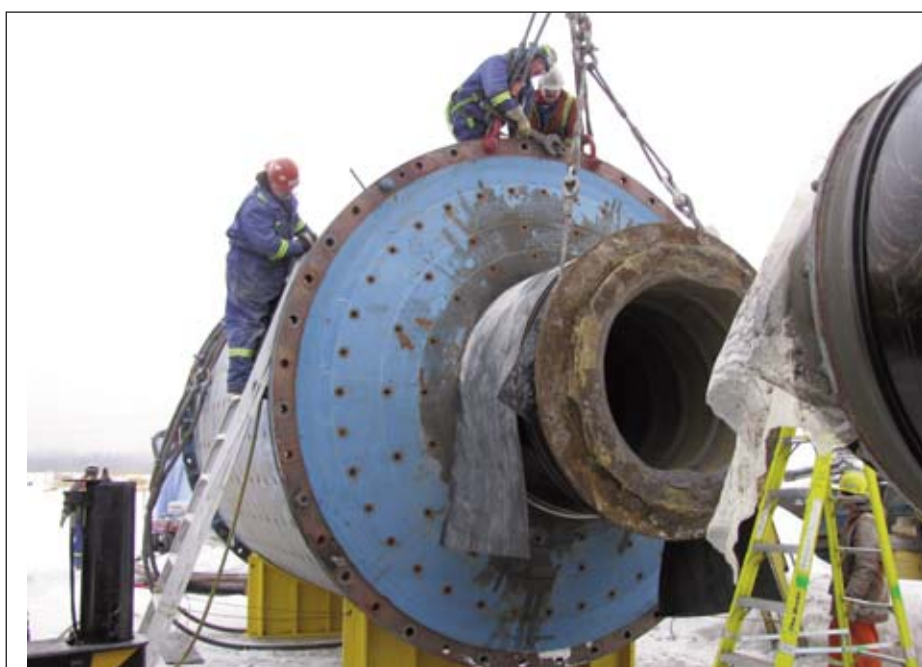
In 2006 and 2008, Fortune purchased all of the buildings, equipment and an inventory of spare parts from the former Golden Giant Mine at Hemlo Ont., intending to relocate it to the Nico Project in Northwest Territories. Here, workers reassemble one of the ball mills at Golden Giant for storage and eventual relocation to the Nico mine site.
