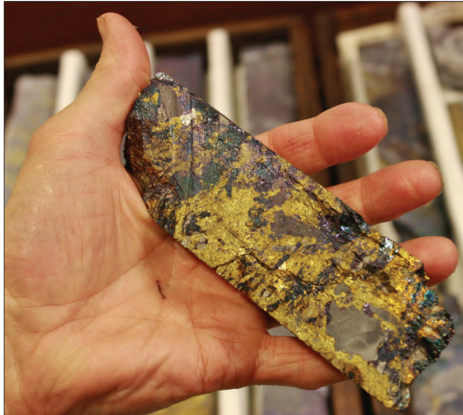
This core is from RC11-187, which cut 178 meters averaging 4 percent copper, including 34.7 meters averaging 12 percent copper at NovaCopper's South Reef target in Northwest Alaska. NovaCopper plans to spend about C$16 million in 2013 exploring South Reef and other targets at the Upper Kobuk Mineral Project.
