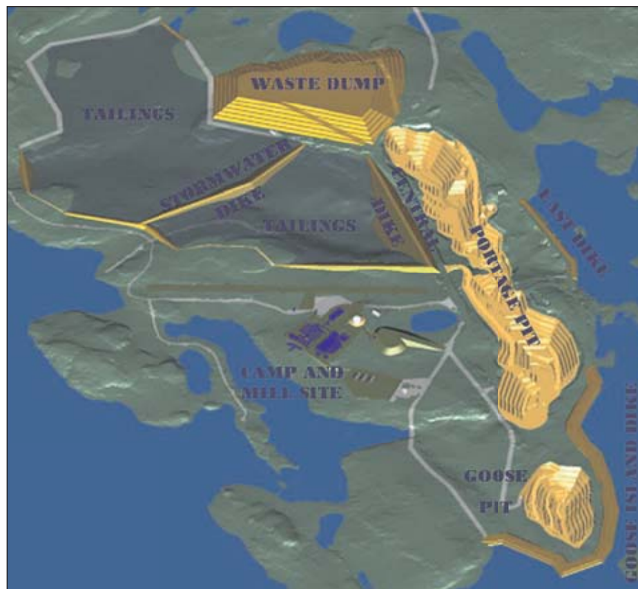
The 11,000-metric-tons-per-day Meadowbank gold mine located in central Nunavut is mined from three low-lying open pits with the aid of water retention dykes.
