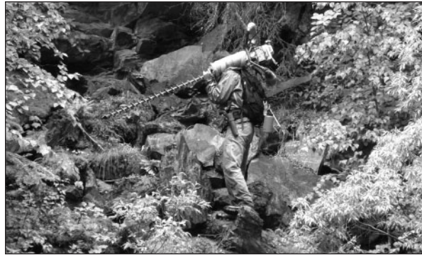
Armed with a handheld auger, a technician makes his way to the next soil sampling site during Contango ORE's 2012 program at the Tetlin gold-copper-silver project in Eastern Alaska. The Texas-based explorer has budgeted US$500,000 for additional reconnaissance exploration in 2013, including soil and rock sampling.
