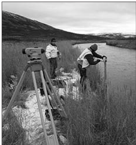
Environmental consultants measure winter stream flow levels near an exploration site at the Pebble copper-gold-molybdenum deposit in Southwest Alaska. This is part of some US$150 million of environmental research carried out by the Pebble Partnership in preparation for permitting.
