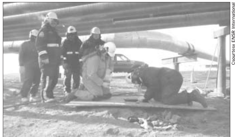
Confirmation sampling on a spill cleanup site at a North Slope facility.
