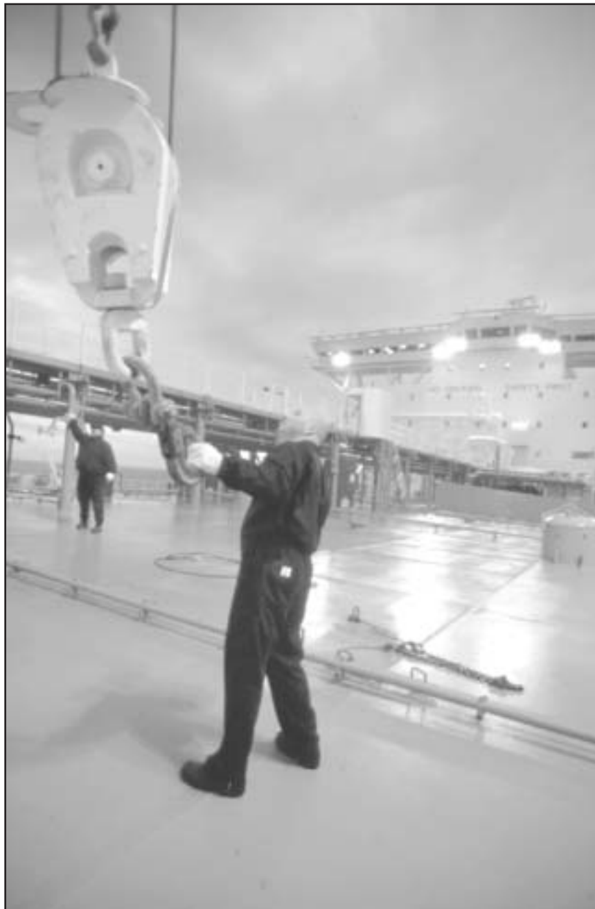
VALDEZ—The deck of the Polar Endeavour. The tanker has 12 cargo tanks which have a combined capacity of just over 1 million barrels.
