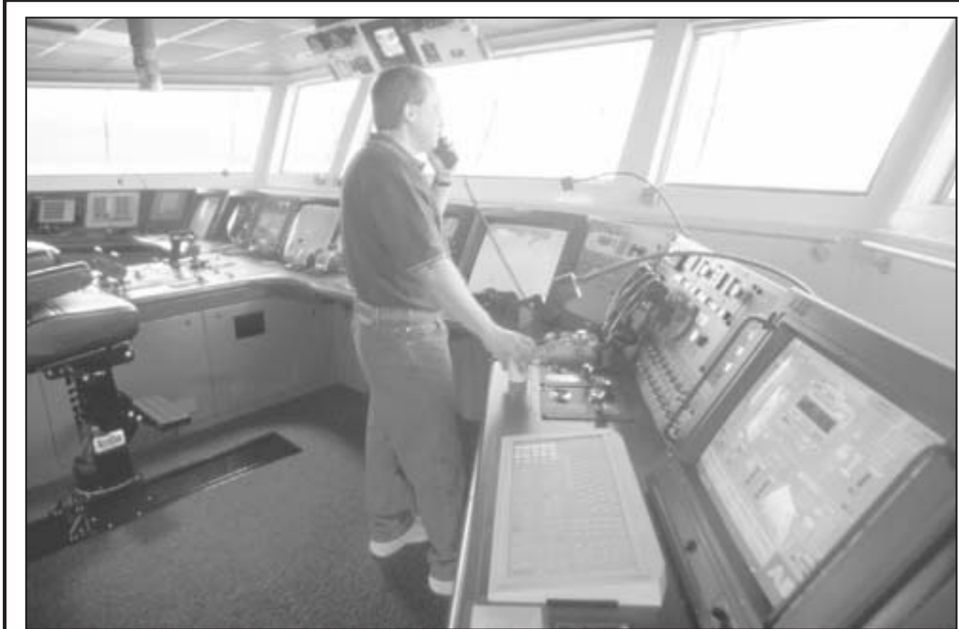
VALDEZ —The bridge of the Polar Endeavour. A control stick actuates the propellers, rudders and bow thruster in one movement of the operator's hand instead of requiring four or five separate commands.
