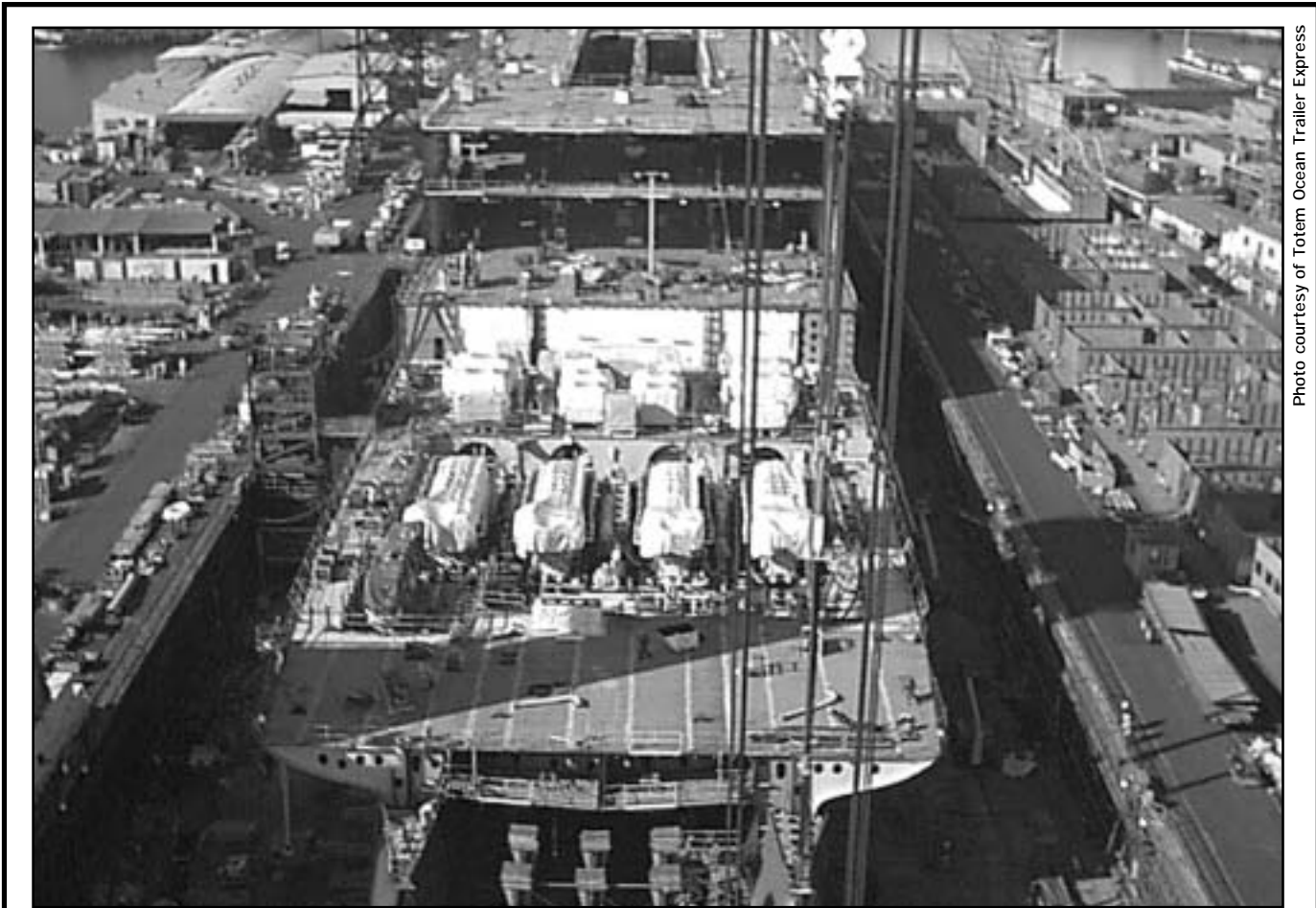
SAN DIEGO — This is the latest photo of Totem Ocean Trailer Express' new Orca class vessel, the Midnight Sun , under construction at National Steel and Shipbuilding Co., Nassco, in San Diego, Calif. This is a shot from the new cranes looking down at the aft end of the ship taken on Feb. 6. Visible in the photo are the Midnight Sun 's four main diesel engines, one auxiliary diesel engine, propulsion and service transformers, and the service switchboard. Also notice the port and starboard stern castings are in place. Upon completion of the Midnight Sun in July 2002 and a second Orca class vessel, the North Star , approximately six months later, Nassco will begin construction of BP's new Alaska class double-hulled tankers.
