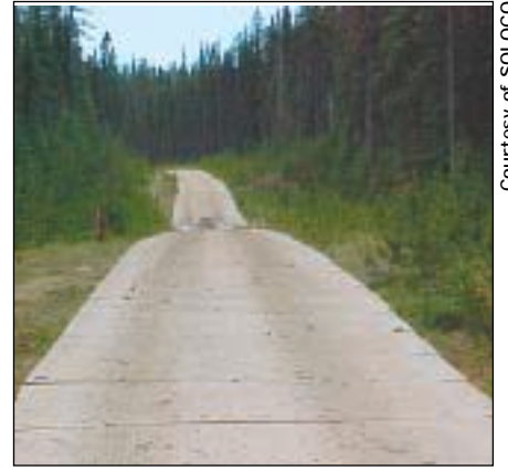
Mats minimize the impact to the natural landscape with DURA-BASE utilization. The mats measure 8 feet by 14 feet and are designed with overlapping lips that combine with a drop-in locking pin to bind the entire mat system together into a solid surface for roads, operational pads and staging areas on soft sub-grades.
