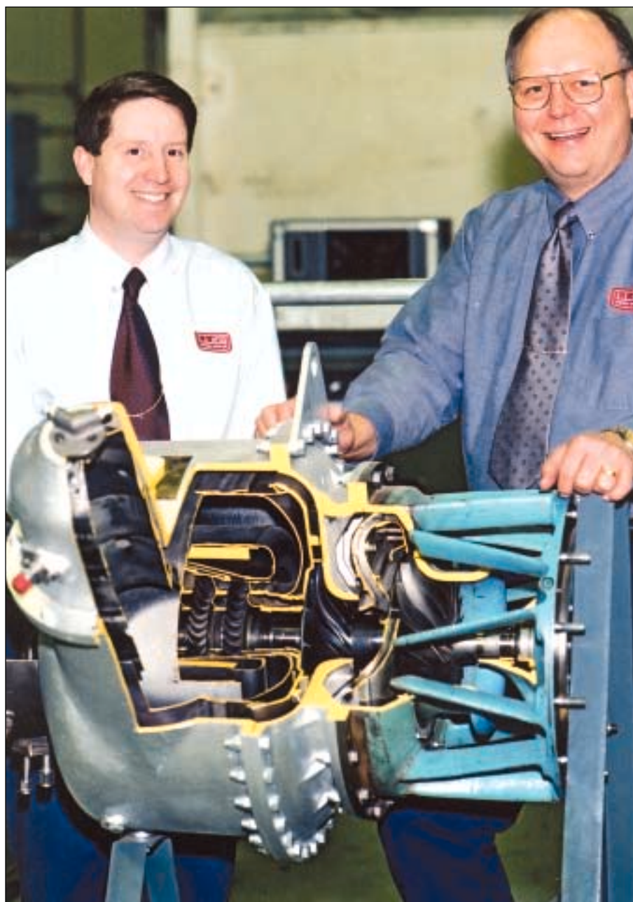
Martin Bellerive and Jim Steel with a cutaway of a Garret ASMES8 engine, one of several engine types supported through Wood Group Alaska.
