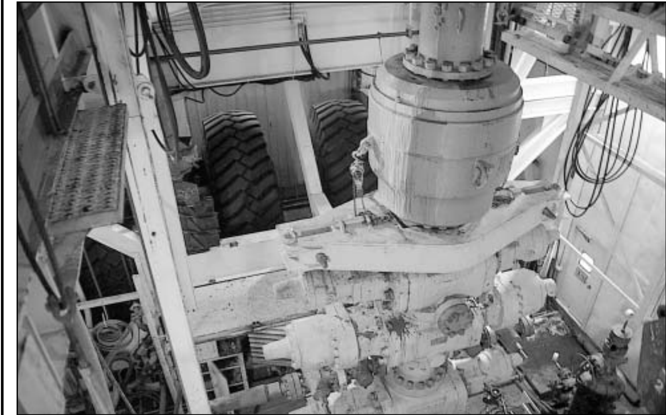
NORTH SLOPE —Pictured here are the tires on Doyon Drilling Inc.'s Rig 19. The mast hoisting capacity of this rig is 1 million pounds with a 12 line hook up. The cantilevered drill floor is capable of a simultaneous combined load of 600,000 pounds for pipe set back, and 900,000 pounds rotary table load.
