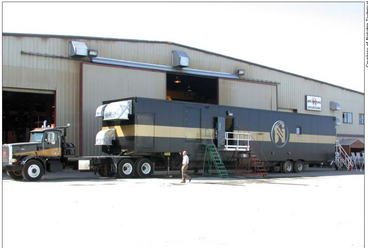
One unit, the Millennium Test Separator, is built into one 80-ton, 70-foot trailer that can be pulled by a truck. The MTS is designed for in-field well testing and is currently being transported to Prudhoe Bay where it will work for BP.
