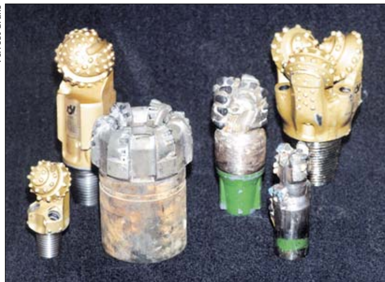
RBI Mono-Cone bits offer additional features not found in other slim hole bits. The cone and bearing capability are significantly larger than a three-cone bit, increasing ROP as well as bearing life.
