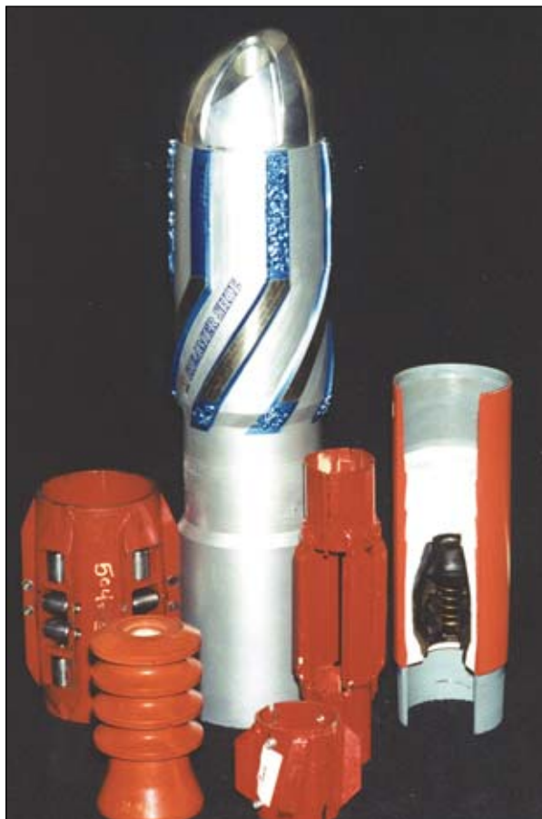
Weatherford Gemoco is the world's leader in casing accessories and offers a wide line of quality centralizers and float equipment for primary cementing needs. Pictured are the Reamer Shoe for reaming through ledges and bridges while running casing, a cutaway of a float collar featuring the PDC drillable SS3 spring-loaded poppet valve recommended for horizontal or deviated wells, and a LoTorq Roller Centralizer used in extended-reach wells to help in torque and drag reduction.
