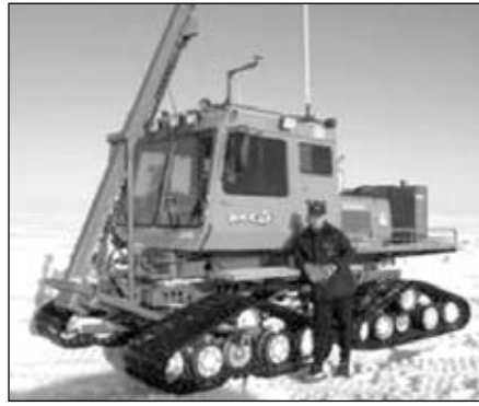
Rubber tracked 2000 < 1 PSI differential steering
