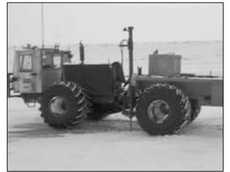
Rubber Wheeled 1997 - 1999 2 PSI articulated steering
