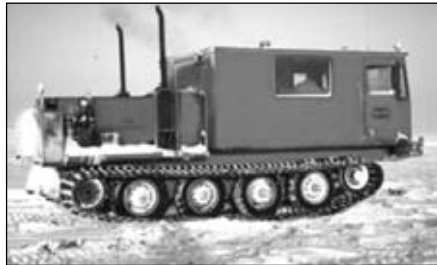
980's to 1999 3 PSI - Steel tracked skid steering
