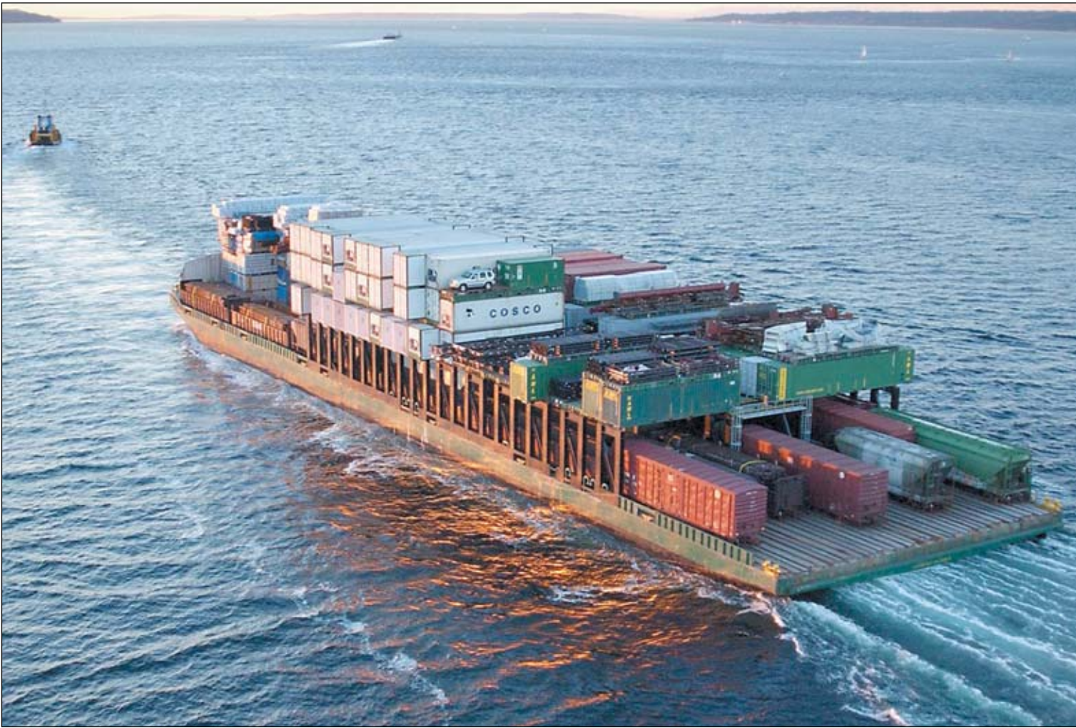
The newest addition to the Lynden group, Alaska-Railbelt-Marine provides rail barge service and regularly scheduled service between Seattle and Whittier. Three new upgraded barges feature overhead racks to allow additional cargo above the rail cars.
