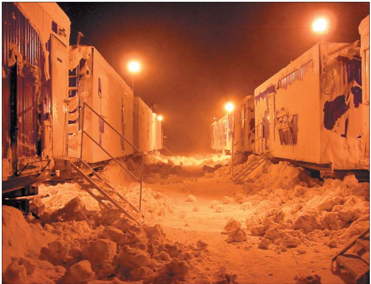
Travco's 85-person custom seismic sleigh camp fabricated for PGS Onshore Inc. The mobile camp trains are completely self-sufficient, including kitchen, showers, lavatories and recreation center.
