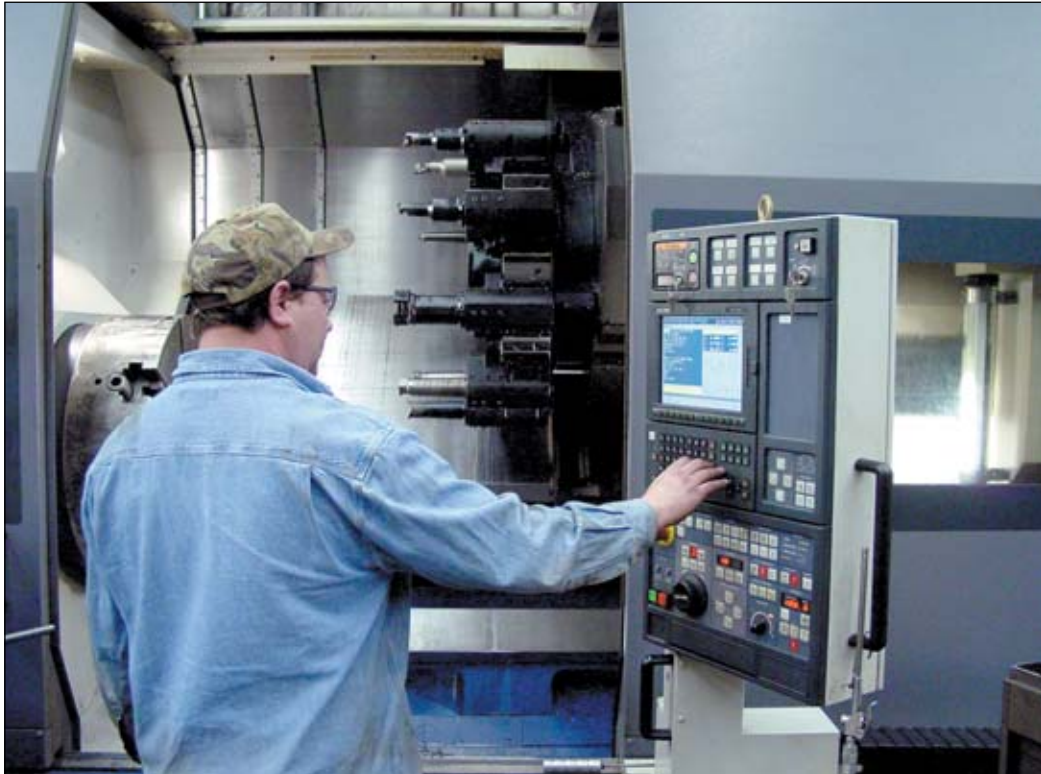
At left, Chris Shumate programs the MoriSekai SL-603 four-axis, computer numerically controlled lathe to machine a UMI Cementrailzer™. Above, Ken Bystedt, owner and founder of Unique Machine Inc.
