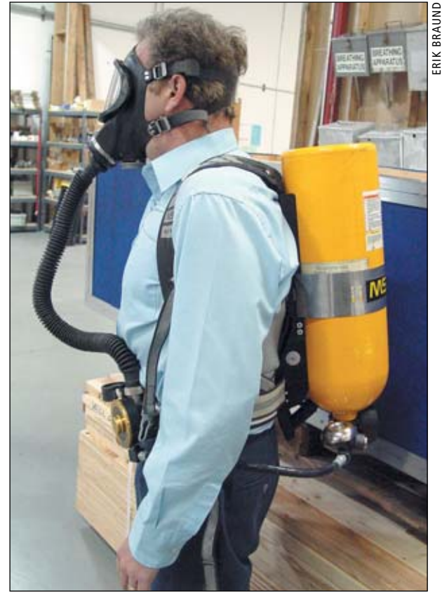
A 30-minute self-contained breathing apparatus. Well Safe sells, rents and services many types of self-contained breathing apparatuses and provides quantitative fit testing on the customer’s location at the Well Safe facility.
