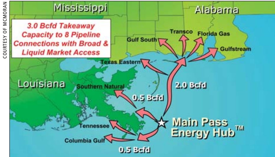
McMoRan's proposed Main Pass Energy Hub would serve both as an offshore liquefied natural gas port and gas storage and delivery system.
