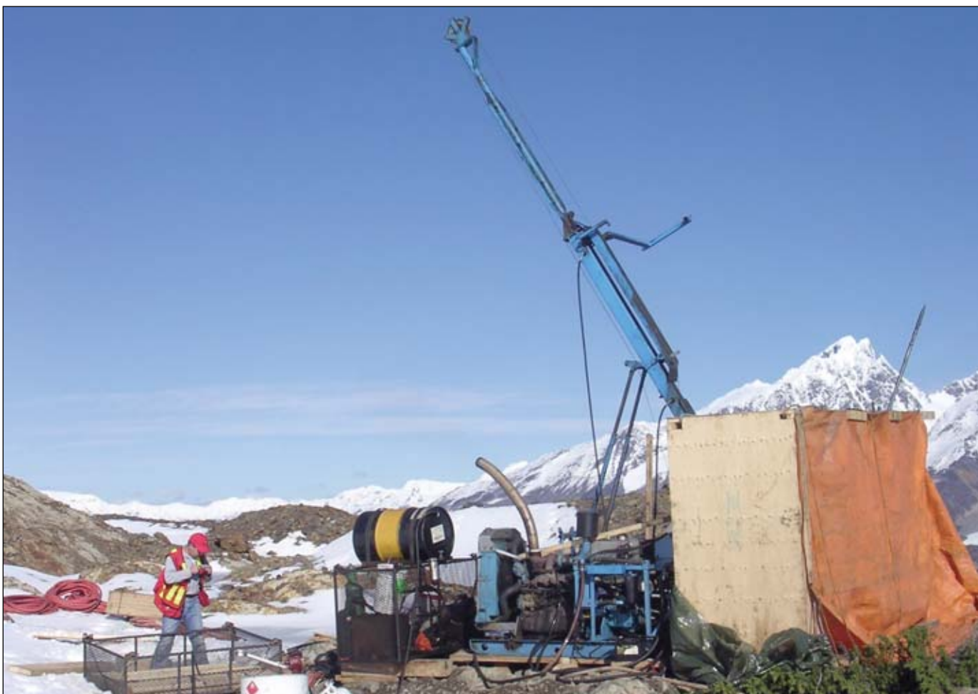
Driftwood Diamond Drilling's rig drilling TIDE-04-03 at the 36 zone. Looking east-northeast.
