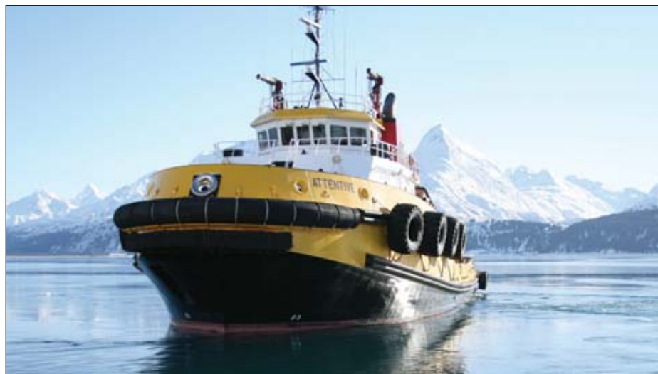
The 10,200-horsepower Crowley prevention-response tug Attentive is one of five state-of-the-art, ocean-class tugs used to escort tankers through Prince William Sound, on their way to and from the Valdez Marine Terminal.
