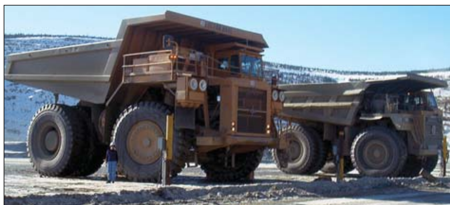
A 200-ton diesel over electric haul truck, the newest in the Fort Knox fleet, dwarfs the mine's 150 ton trucks. The company plans to purchase six more haul trucks and another loader in order to handle waste rock.
