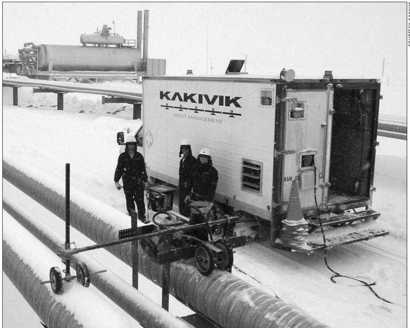
Kakivik workers monitor the Real Time Radiography testing unit.
