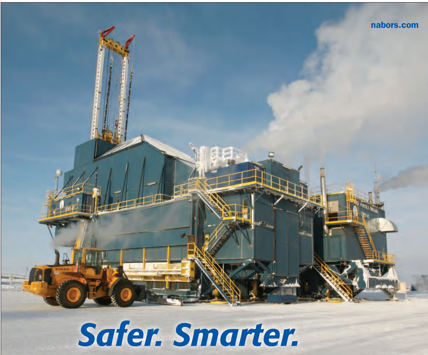
Huge new land rig coming: BlueCrest Energy is bringing in a rig to develop the Cook Inlet oil accumulation, using extended reach wells drilled from onshore. The derrick, which will hold simultaneously 24,000 feet of drill pipe, is pictured here on March 18 in front of the factory in Liberty, Texas. The company has already started shipping rig components to Alaska. It will require 115 large truckloads.
