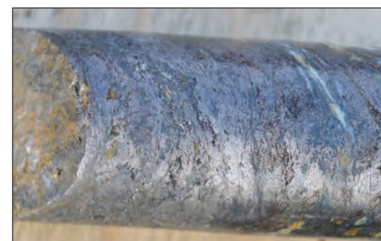
A section of massive graphite cut during the 2013 drill program at the Graphite Creek project near Nome, Alaska. Graphite One Resources is now working out the process of producing the spherical graphite used as anode material in the lithium-ion batteries that power electric vehicles and other mobile electronic devices.
