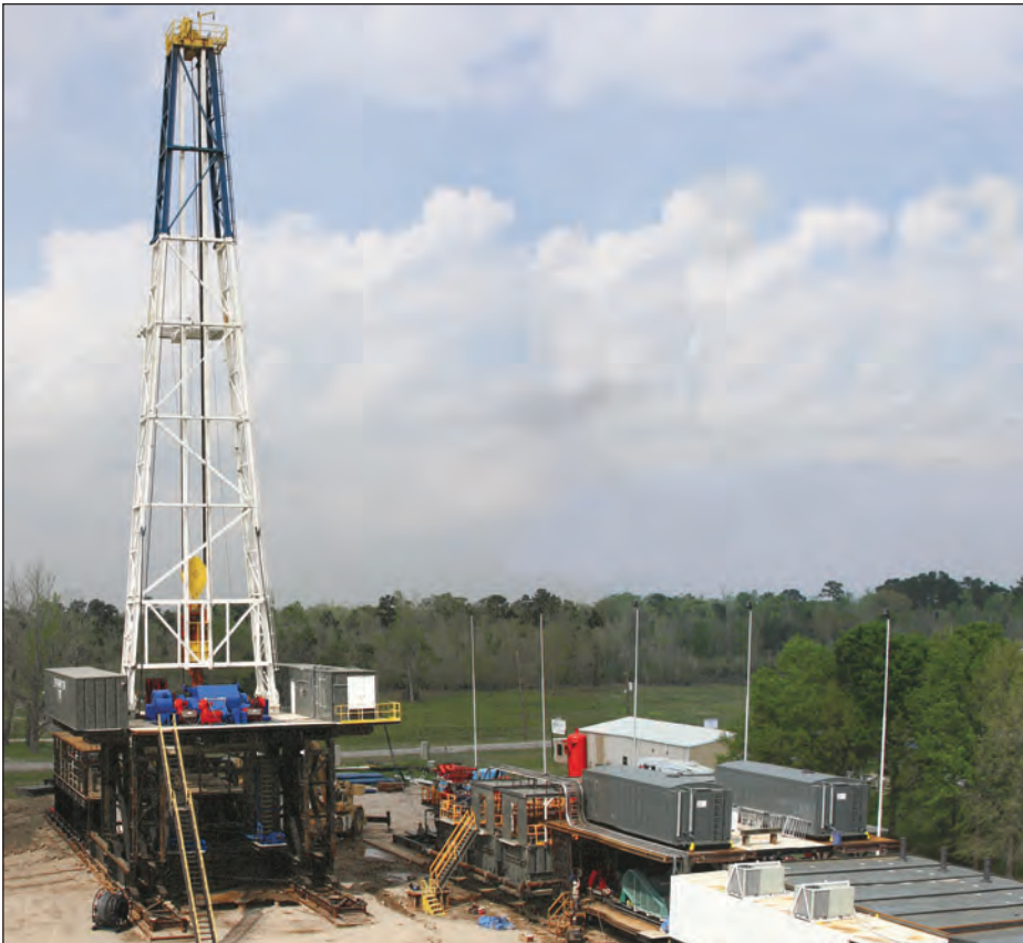
Huge new land rig coming: BlueCrest Energy is bringing in a rig to develop the Cook Inlet oil accumulation, using extended reach wells drilled from onshore. The derrick, which will hold simultaneously 24,000 feet of drill pipe, is pictured here on March 18 in front of the factory in Liberty, Texas. The company has already started shipping rig components to Alaska. It will require 115 large truckloads.
