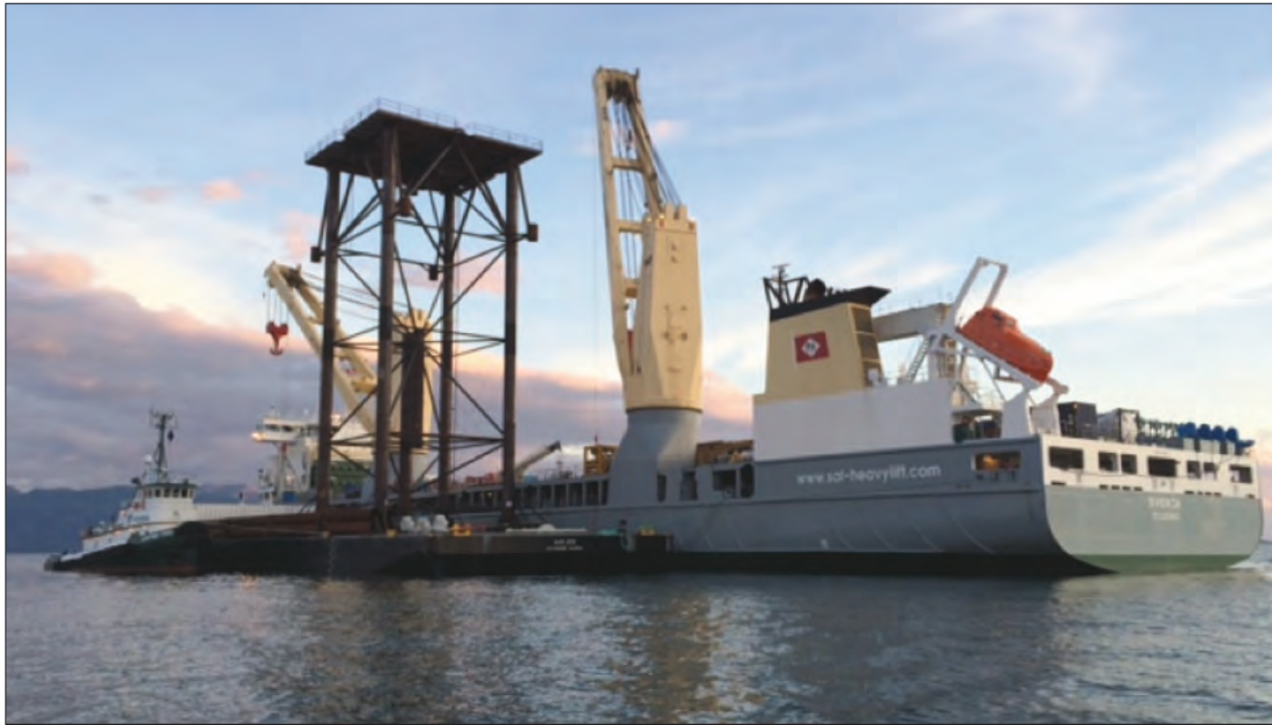
Heavy lift ship MV Svenja with template to be set at Kitchen Lights unit KLU Platform A
