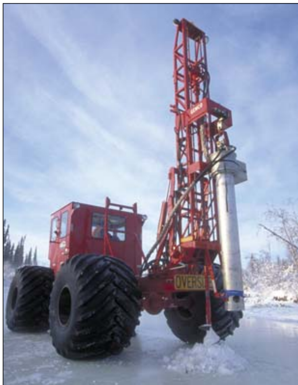
Above, this year's 47-mile Teck-Pogo mine winter road built by Cruz crews in less than 30 days did not go without accolades. Pictured is work on a bridge. At left, a Cruz Construction ice auger.
