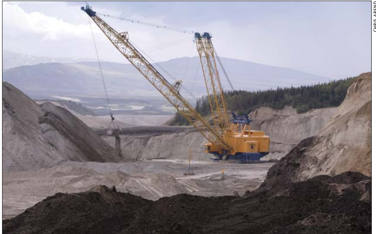
The Bucyrus-Erie 1300W walking dragline at work removing overburden in Two Bull Ridge Mine, Usibelli Coal Mine
