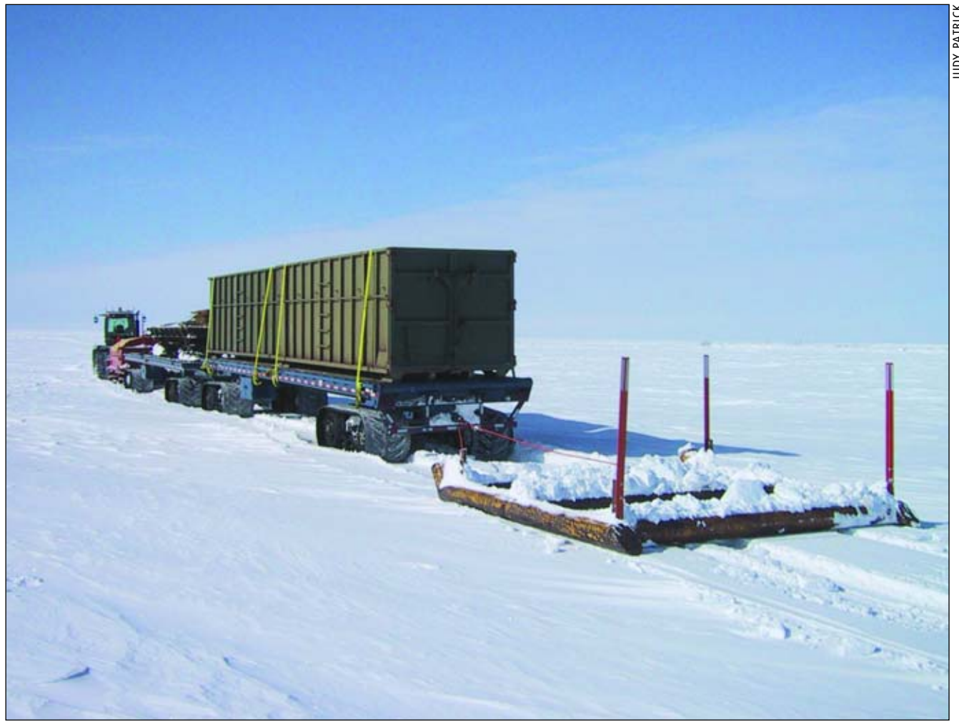
Last spring when Western GECO discontinued work in Alaska, Cruz Construction purchased its assets, including tundra-approved ATV trailers and power units capable of hauling 30-ton loads as well as some Tucker Sno-cats. See the company profile on page B13.
