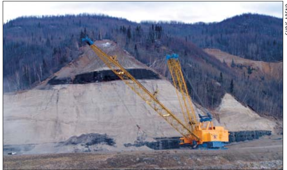
A Usibelli coal dragline at work
