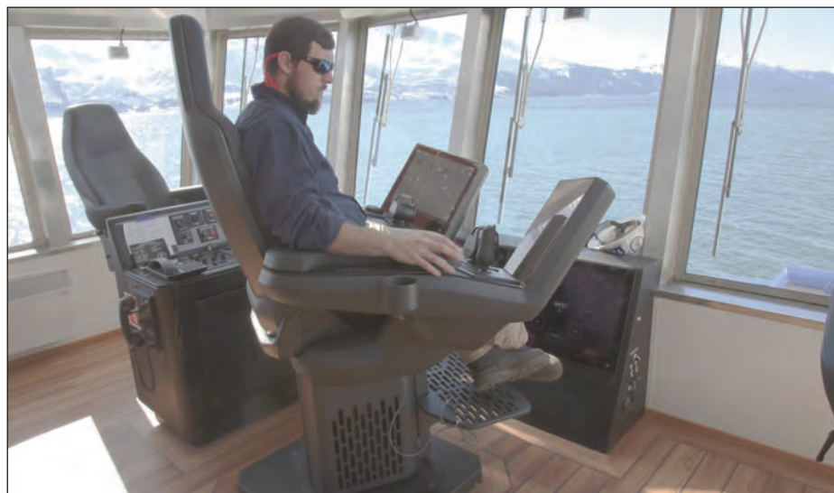
The high-tech bridge of the Commander escort tug has electronic controls that enable the huge vessel to be precisely maneuvered, together with display screens that show maps and other information.
