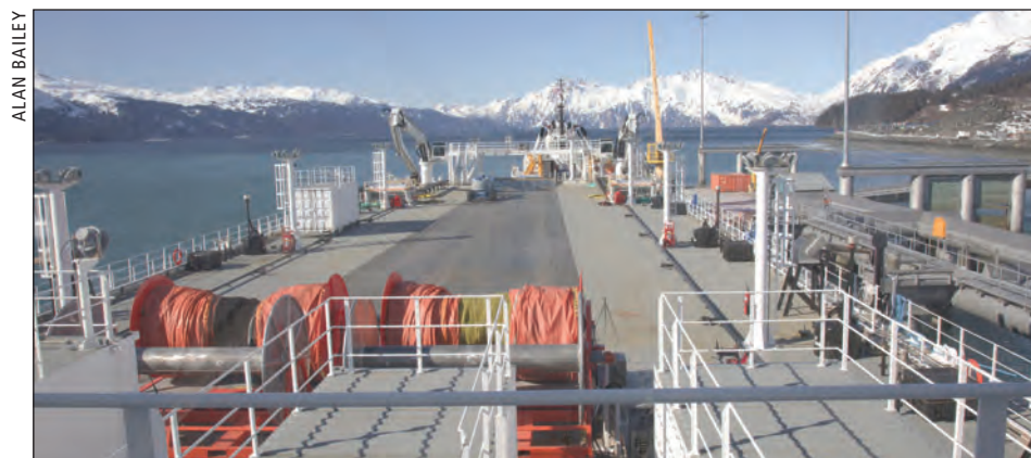
The deck of the new OSRB-1 response barge is long enough to allow the inflation of complete twin lengths of boom, before sliding the boom into the water.
