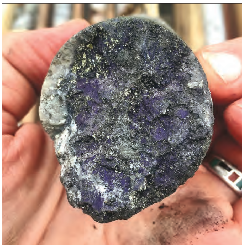
This chalcocite copper mineralization was encountered about 135 meters down hole RT-11, which was drilled about 22 meters south of RT-7, the last hole Anaconda drilled at Round Top in the early 1980s.
