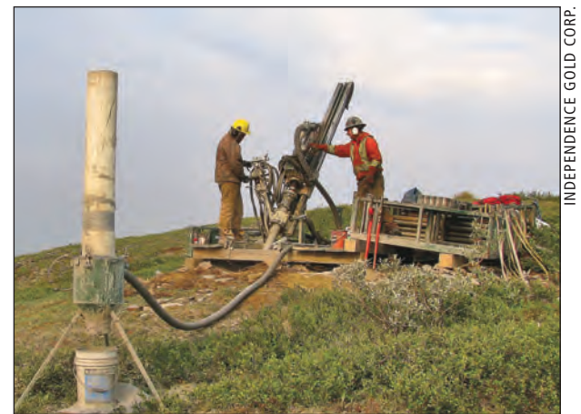
Part of Independence Gold's 2,000-meter reverse circulation drill program at Boulevard will follow up on a 2015 hole that cut 4.25 grams per metric ton gold across 6.1 meters at the property's Denali zone.
