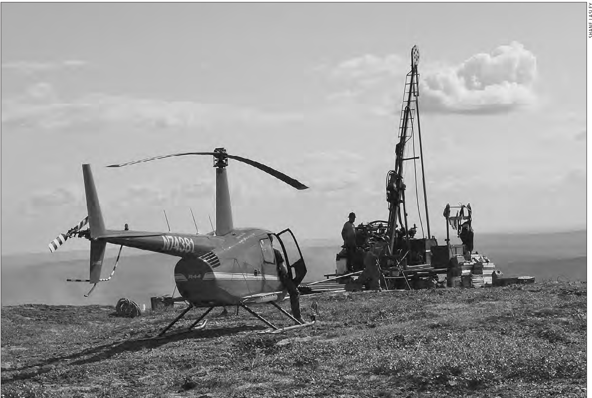
By July 15, crews were on the fourth hole of a roughly 1,500-meter drill program at Round Top. Mounted on tracks, this rig being leased from More Core Drilling can be driven to a new drill location and resume drilling in a matter of hours. The short span between holes, combined with requiring a much smaller support helicopter primarily for transport of core and personnel, is keeping Western Alaska Copper & Gold's drill costs low.
