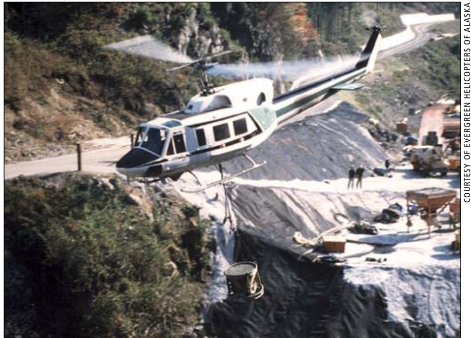
Mineral exploration and development in Alaska is clipping along at a pace not seen in more than five years. In the process, finding available aircraft has been tough. Pictured is an Evergreen Helicopters Bell 212 lifting a bucket of concrete during work at a mining site.
