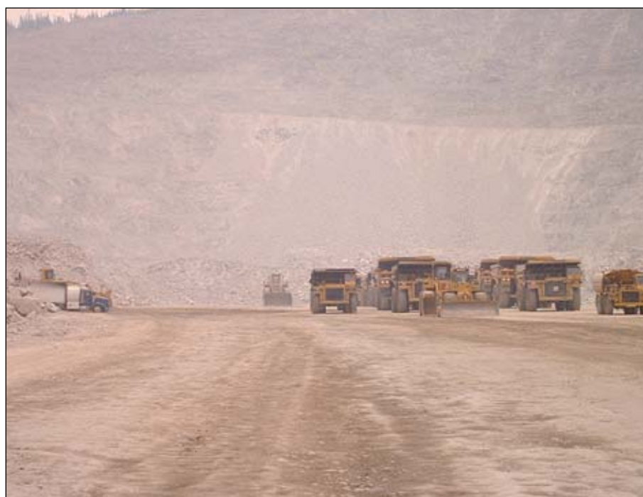
All of the "rolling stock" of large earthmoving equipment was moved and parked at the bottom of the pit, potentially protecting the equipment from fire and keeping it consolidated in case fire crews needed to use the mine site
