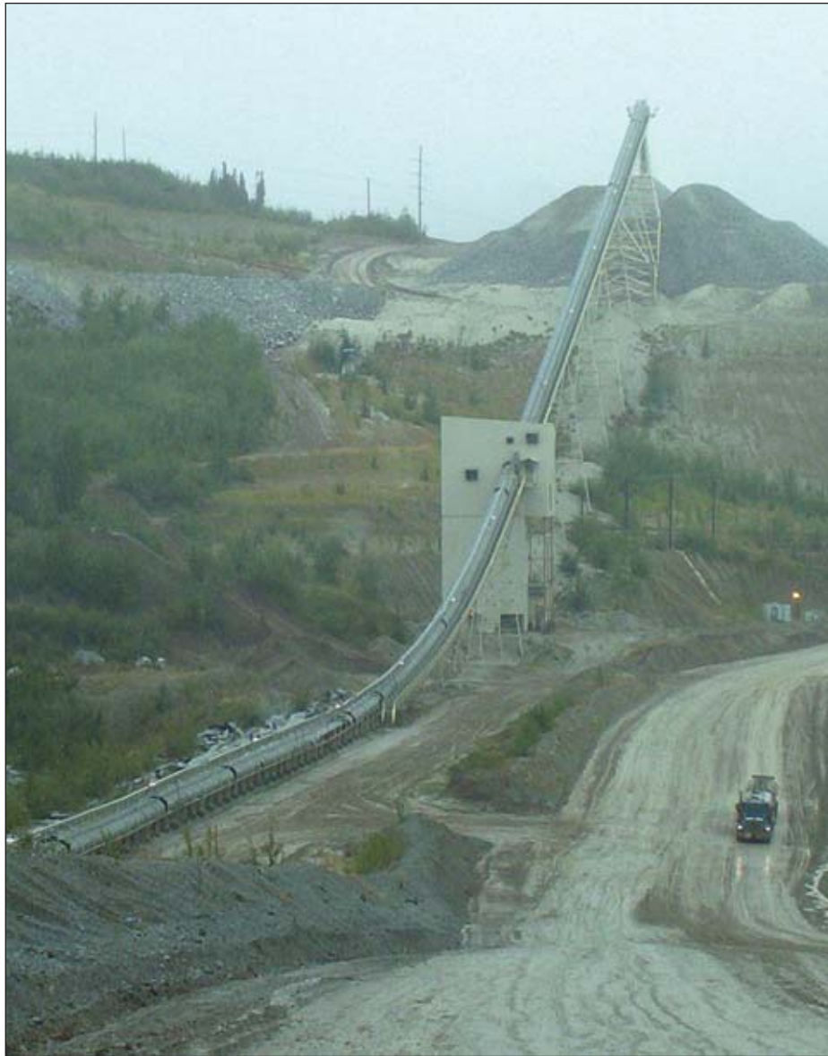
Ore is transported half a mile by conveyor belt from the crusher to the stockpile
