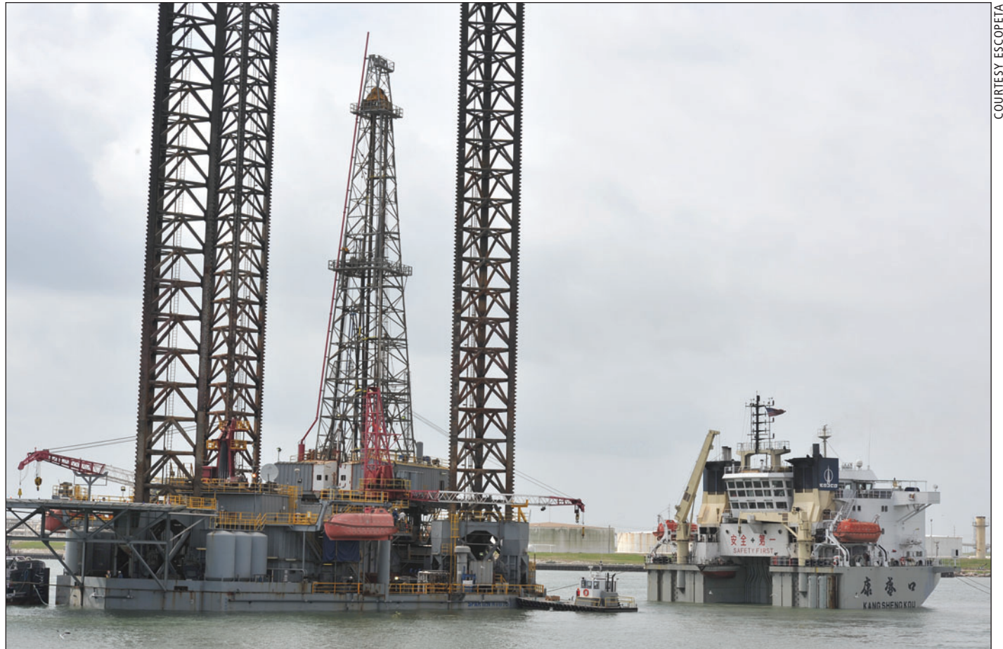
Escopeta's Oil's Spartan 151 jack-up was loaded on a heavy lift vessel on March 13 for its trip north to Alaska's Cook Inlet. The stern is pictured above, with the rig sitting on the submerged deck of the vessel.
