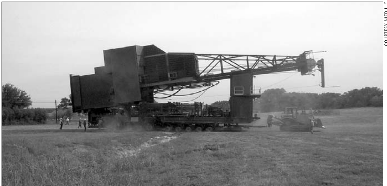
Moving the Arctic Millennium's drill module. The Millennium travels at 10 mph, goes together in 24 hours, and only includes 11 pieces. See the company profile on page C12.
