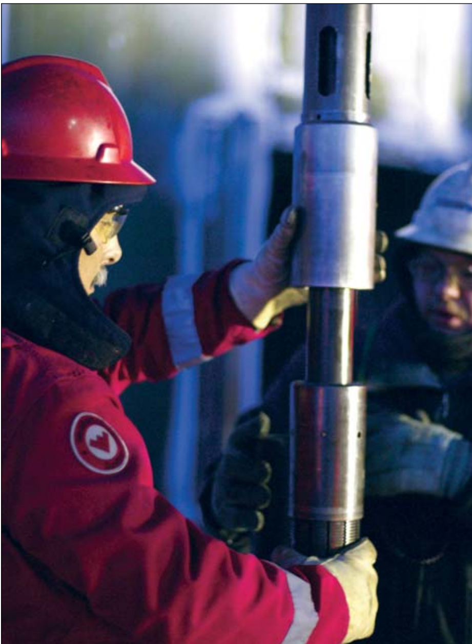
A Schlumberger Wireline crew working with a Weatherford operator to run a mechanical tubing patch.
