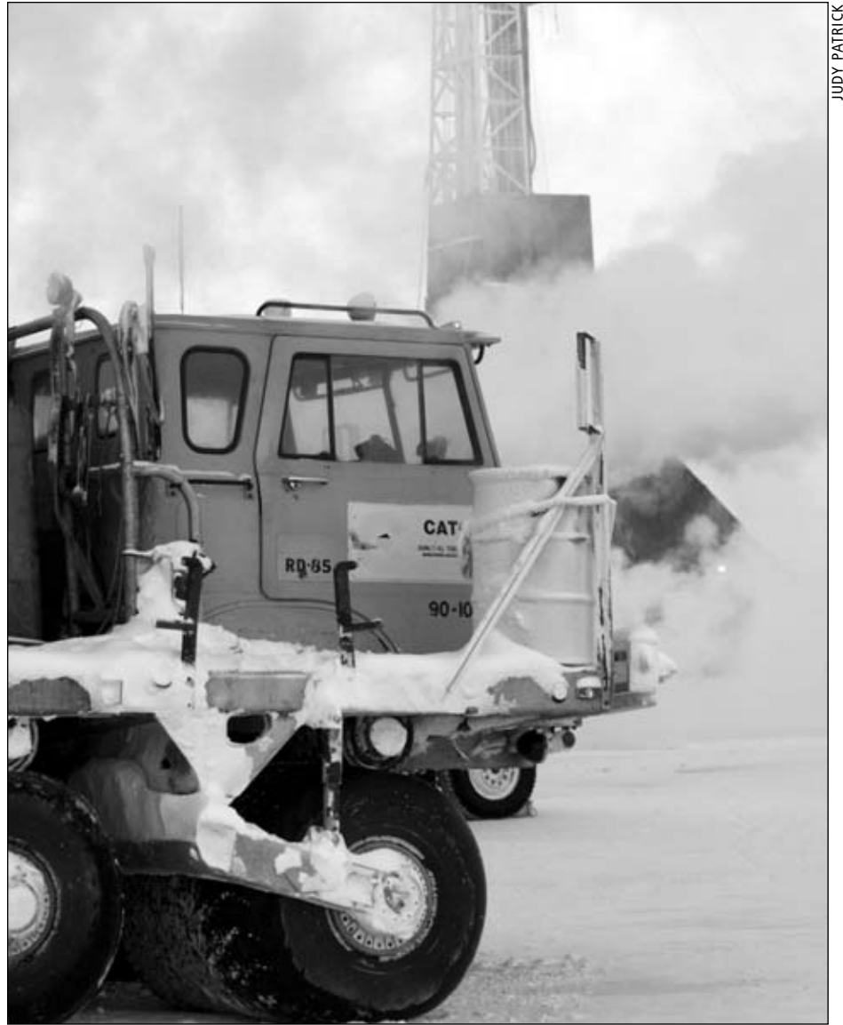
Rolligon at a remote exploration site. The rolligons transported the entire drill rig, camp and all related drilling supplies and equipment to the site.
