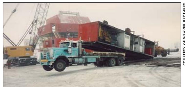
With winches to pull loads on and off, Weaver Brothers trucks can carry more than 100,000 pounds and have proved particularly effective for transporting drilling rigs.
