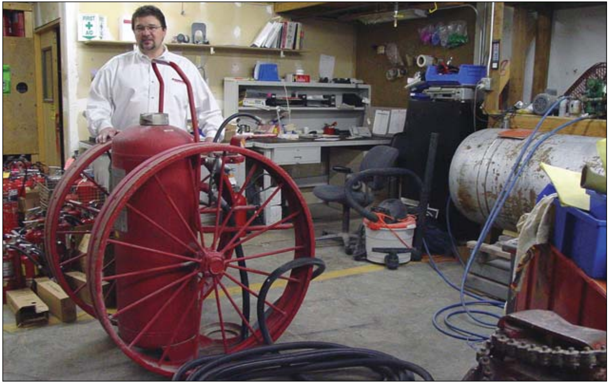
In the extinguisher shop, Engineered Fire and Safety Sales Manager Dale Shirley shows a high-volume, wheeled fire extinguisher, often used at heliports and airports.
