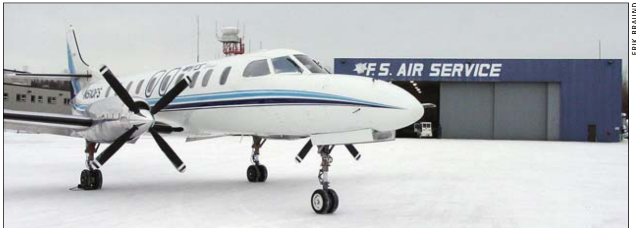
The versatile Metro 23's large rear door is well-configured to haul equipment to the oil fields and other remote locations. F.S. Air is contracted with the Department of Defense to transport people to remote locations, radar sites and military installations. Passenger capacity is 19.
