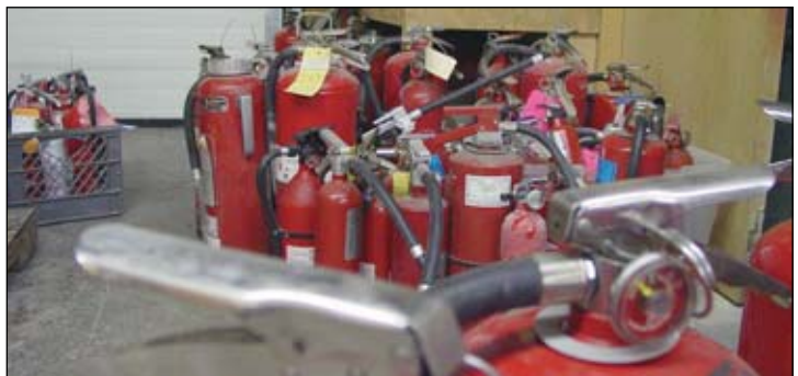
Fire extinguishers of all sizes await recharging in the Engineered Fire and Safety extinguisher shop. The company recharges and hydro tests commercial extinguishers.
