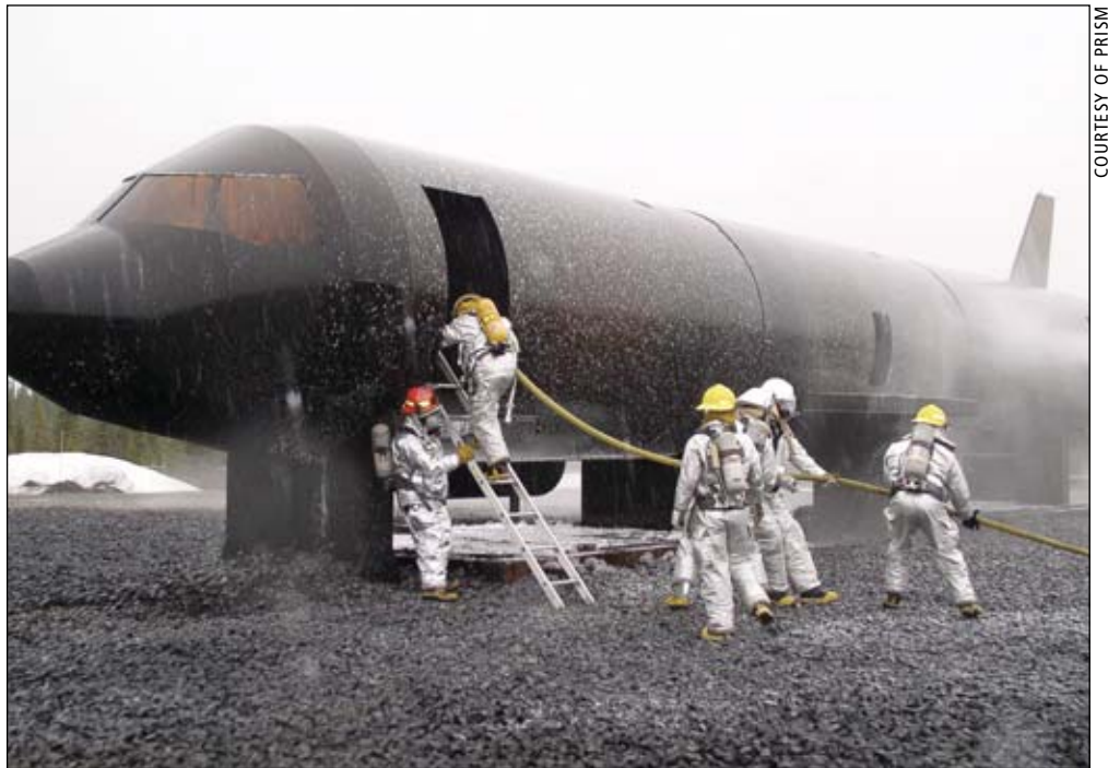
Hot-fire trainers at the PRISM Training Center use propane fueled burners to simulate aircraft fires.
