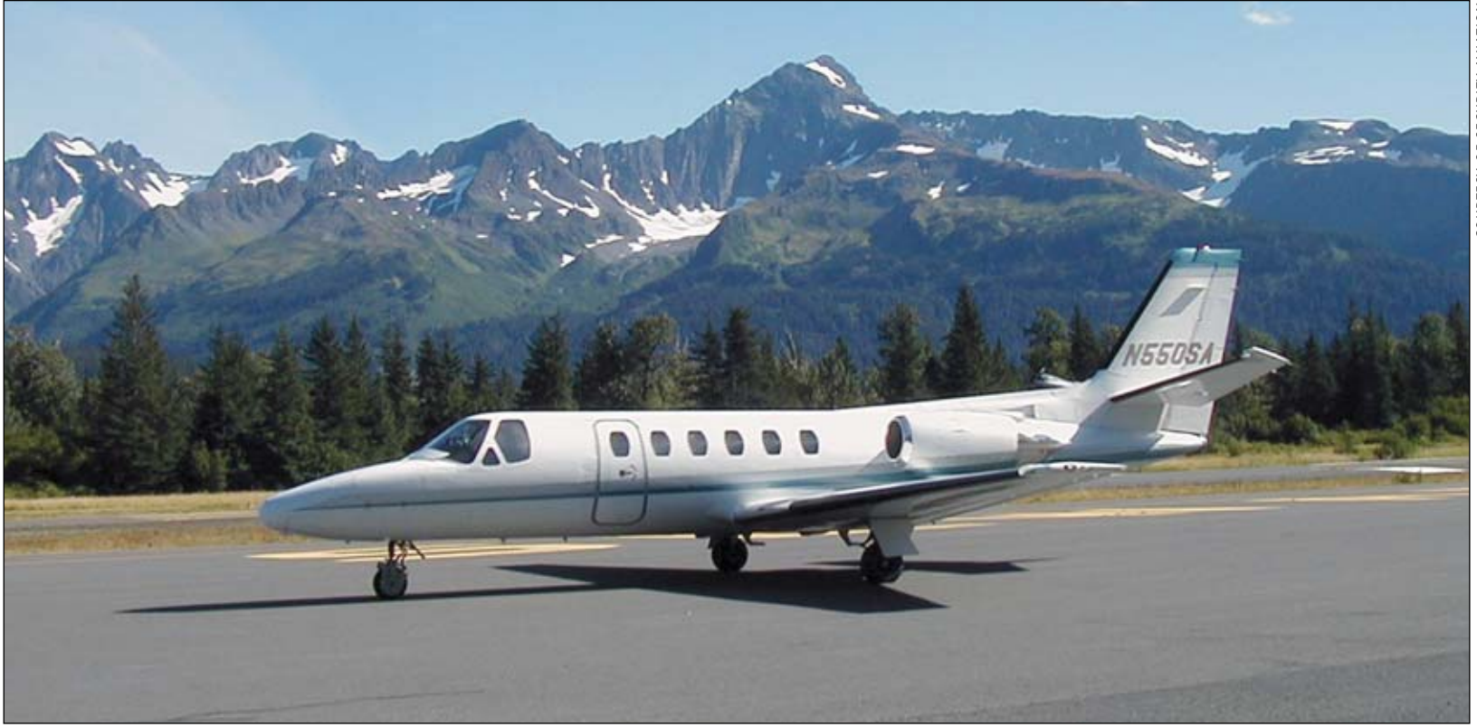
Security Aviation's Citation II jet gets well up above the weather and works well for trips to the Aleutian Chain and Seattle. The straight wing design and gravel kit allow for short runway performance capability.
