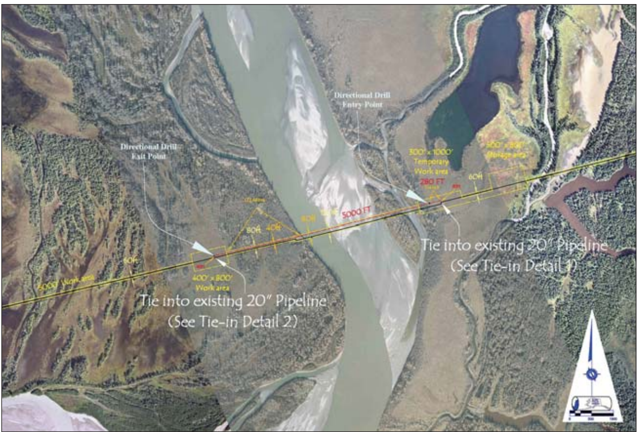
Route of the relocated Beluga pipeline crossing of the east channel of the Susitna River.
