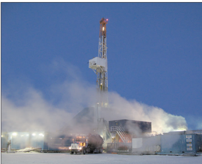
The Calgary-based junior said April 7 that the Langley E-07 well tested at restricted flow rates of 13 million cubic feet per day on a 2-inch choke.
