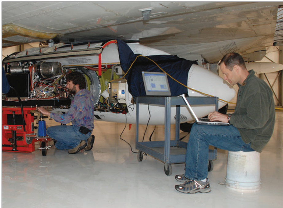
NOAA Earth System Research Laboratory employees David Thomson and Chuck Brock, ARCPAC co-lead mission scientists, with the PALMS (Particle Analysis by Laser Mass Spectrometry) instrument pod.
