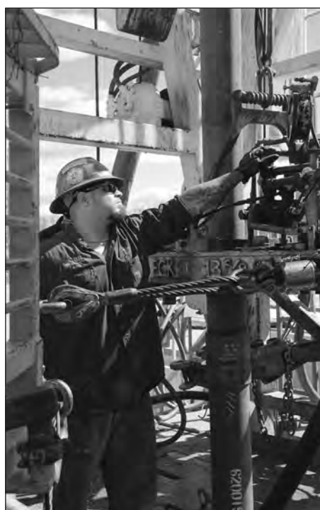
Positioning well casing for insertion into the well bore of Doyon's Toghothle No. 1 well in the Nenana basin.
