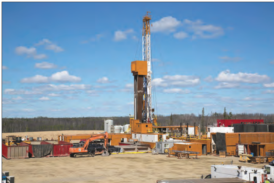
Doyon's Arctic Fox drilling rig on location on a gravel drilling pad, drilling the Toghothle No. 1 well in the Nenana basin, west of the Nenana River.
