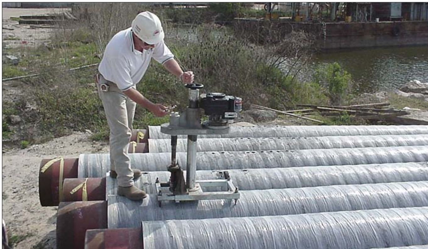
A NACE coating inspector verifying compression test results on concrete coated pipe
