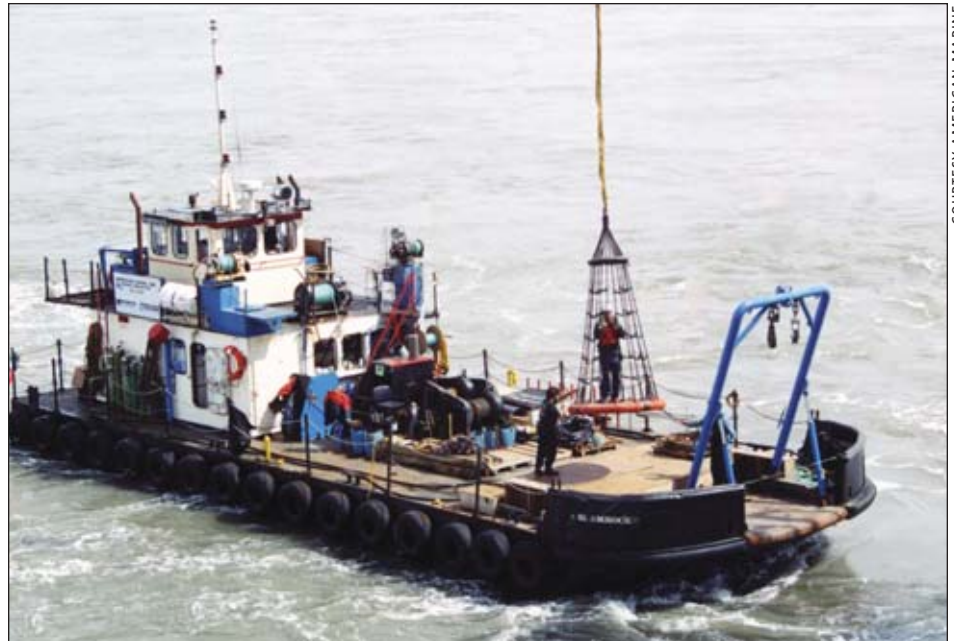
Personnel transfer from Cook Inlet Platform to DSV Shamrock.
