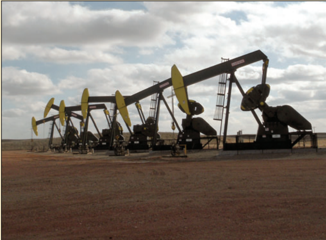
Six Hess Corp. dual-lateral wells in the Ross field approximately six miles east of Stanley in central Mountrail County, N.D. One lateral of each well targets the middle Bakken and the other the Three Forks.
