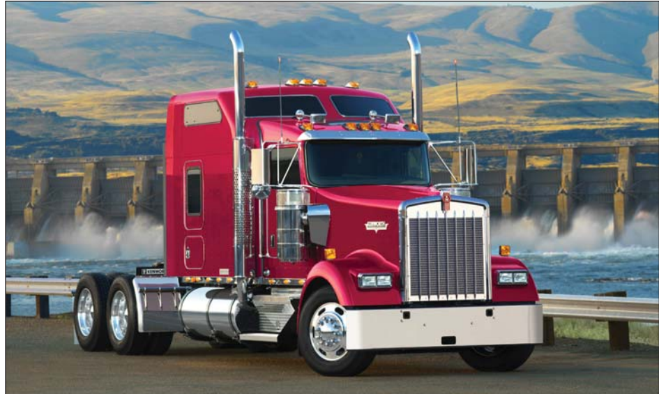
Kenworth's W900L (pictured) and T800 truck models, spec'd with high horsepower engines, heavy rear ends and suspensions, are popular models in Alaska because they can handle the heavy loads haulers routinely pull up the demanding 414-mile Dalton Highway to Prudhoe Bay.
