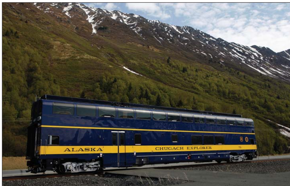
The fuel-efficient all-in-one Chugach Explorer is a bi-level diesel multiple unit built especially for the Alaska Railroad's new Whistle Stop Service to the Chugach National Forest.
