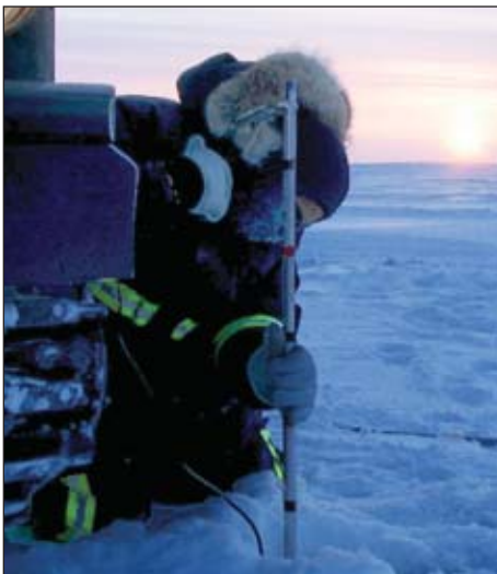
Baker conducts bi-monthly water quality monitoring at the Colville River Ice Bridge. A water resource team member is shown above collecting water velocity measurements under approximately 4.5 feet of ice on the Colville River in February 2005.
