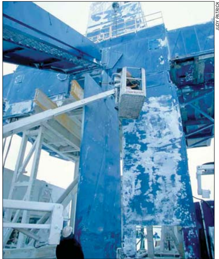
In the first quarter of 2002 Anadarko spud its first Anadarko-operated well on Alaska's North Slope in the National Petroleum Reserve-Alaska at the Altamura prospect. Above, crews attach a 30 foot wind wall to Nabors Alaska Drilling Rig 14 E. The ramp in the upper left contains all power from the SCR unit.
