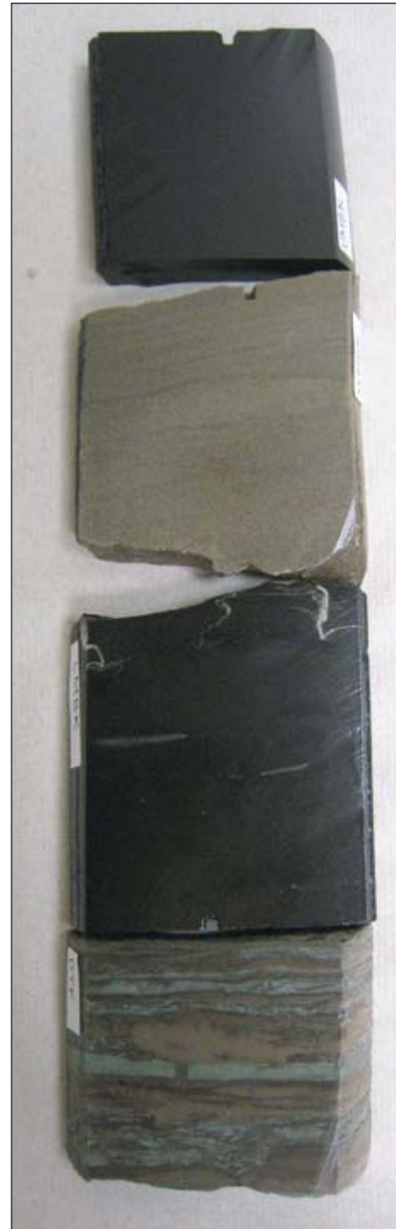
From top to bottom: the upper member (shale) of the Bakken formation, the middle member (dolomitic sandstone reservoir); the lower member (shale); and the upper member of the Three Forks formation, which is a tight variable oil reservoir consisting of green and tan, sometime pinkish, carbonate mudstone, as well as shale but with no organic content.. Missing just above the upper Three Forks is a sandstone that used to be called the Sanish, but is now considered one of the Bakken members, with a new name: Pronghorn.
