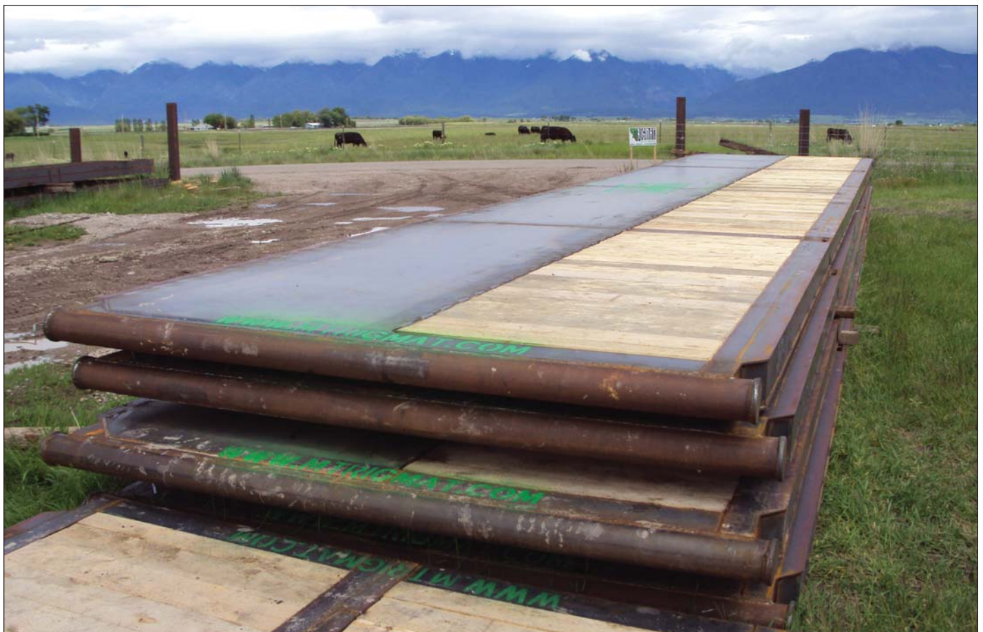
8x40 rigmats with custom steel decking
