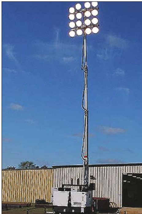
The Magnalight Mega Tower 24000 extends to 50 feet in height, produces 2,400,000 Lumens, and can illuminate over 10 acres.
