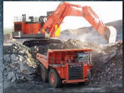
EX1900-6 Excavator and EH1700 Truck at Alaska Gold Company.
