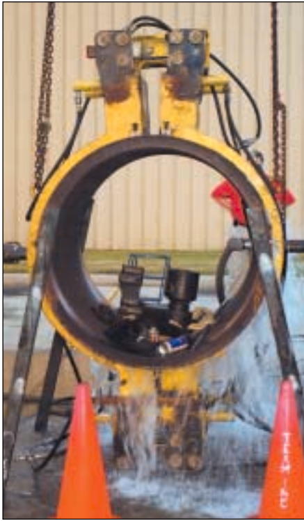
Top right, Oct. 4: Crude oil shoots out of the pipeline after it was punctured by a bullet. Above, fall 2001: Testing the newly designed hydraulic clamp.
