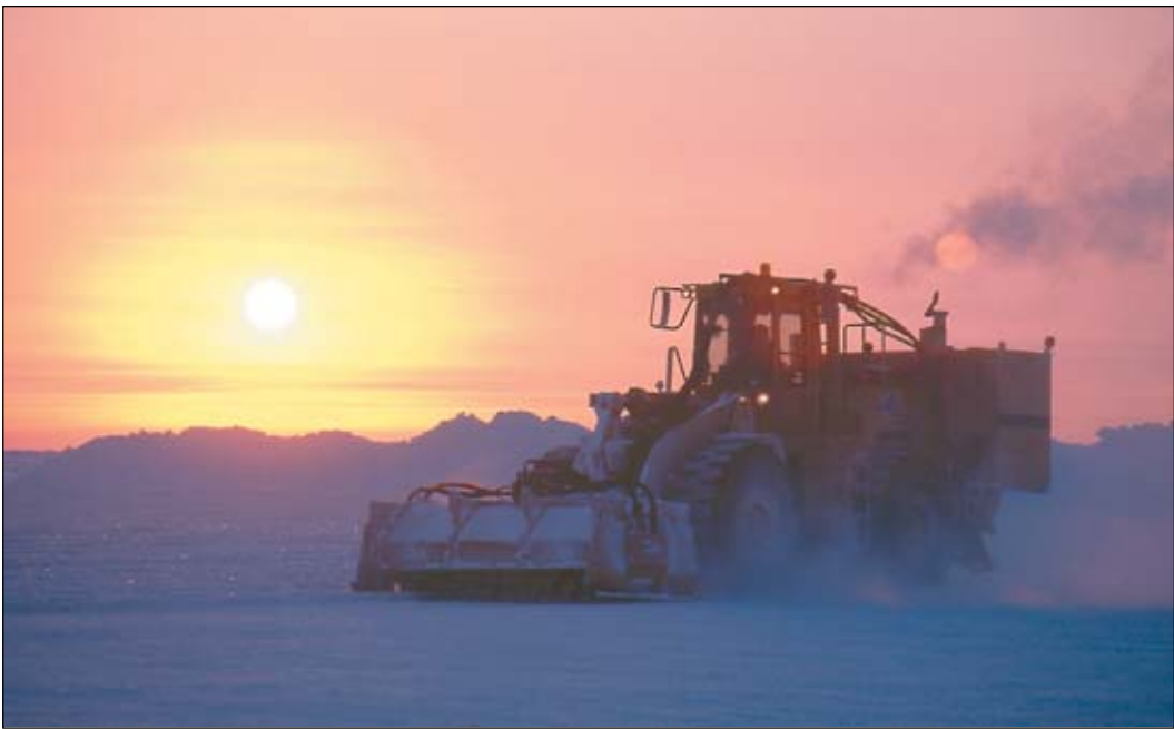
Clockwise from top, Catco's equipment building island for Natchiq well. Alaska Interstate Construction's Trimmer makes ice chips for road and pad construction. Marker stick at Oooguruk indicating that 10 more feet is needed to finish island construction.
