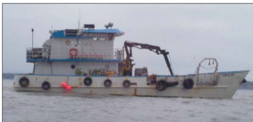
The heart of the company — the Sand Island, Offshore Divers' 72-foot retrofitted dive boat, formerly an offshore rescue and supply vessel. Visible forward of the house are the hydraulic crane and A-frame. A decompression chamber is located under the deck.
