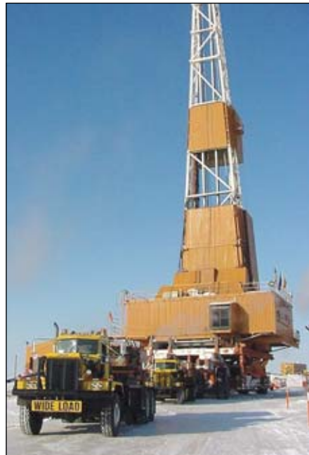
At left, Doyon 19 rig floor on rig floor transporter. Above, moving out: Doyon Drilling rig 19 being moved on rig floor transporter
