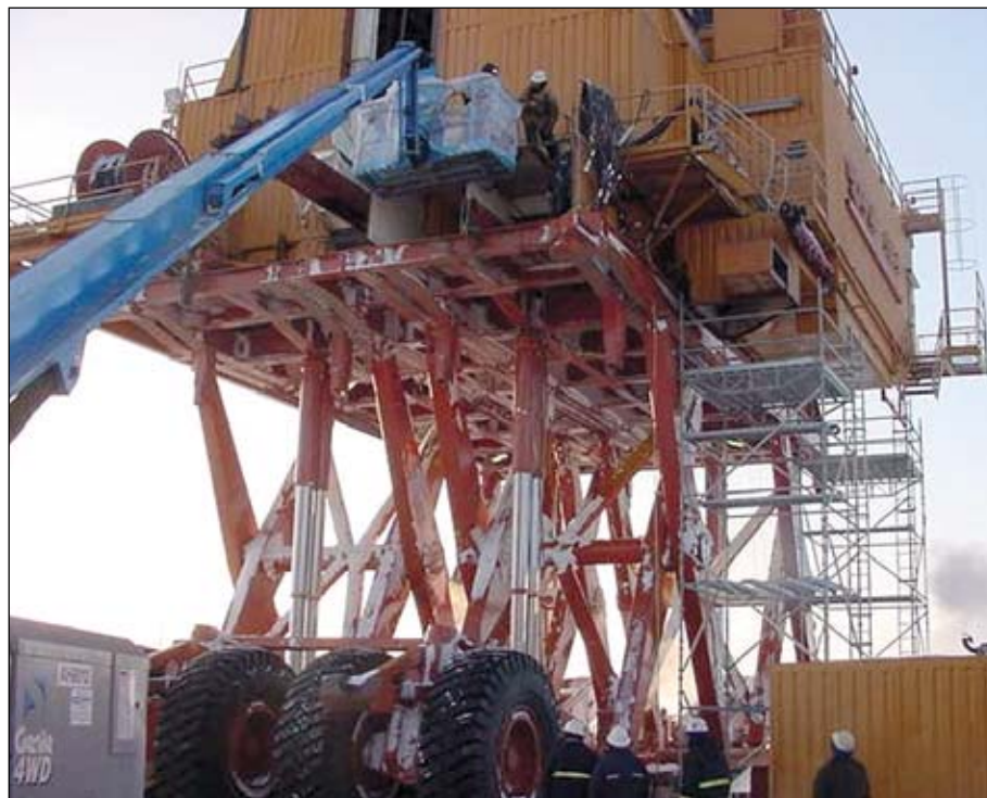
At left, Doyon 19 rig floor on rig floor transporter. Above, moving out: Doyon Drilling rig 19 being moved on rig floor transporter
