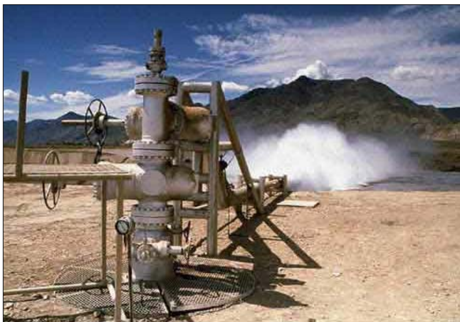
If the well is good enough, a wellhead, with valves and control equipment, is built onto the top of the well casing.
