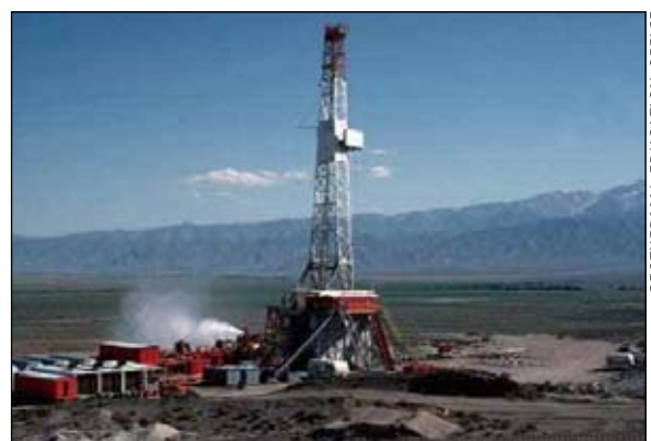
Production-sized wells require large drill rigs like these and can cost as much as a million dollars or more to drill. Geothermal wells can be drilled over two miles deep.
